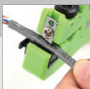
Strip network cable
