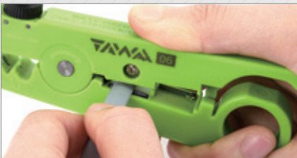
Cut flat line cutting edge
