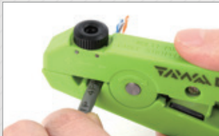
Strip ethernet cable
